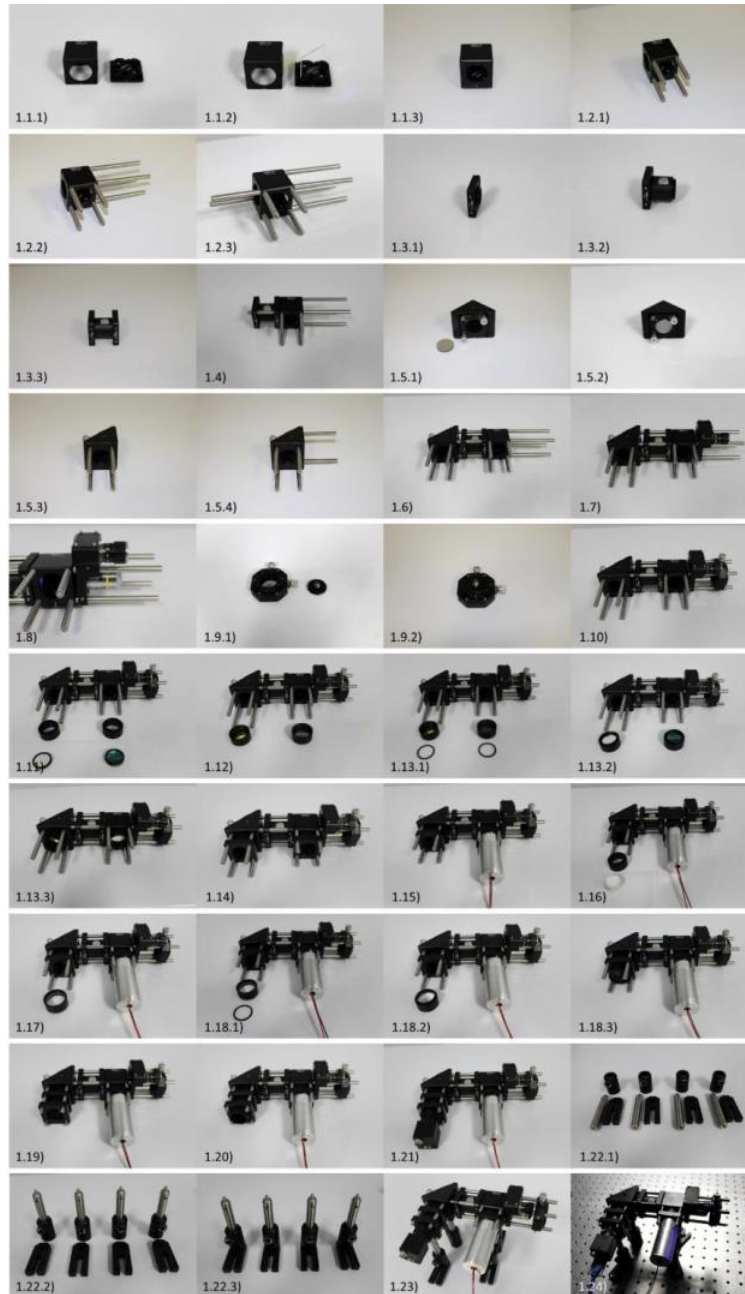
Figure 4. Assembly of the high-resolution fluorescence microendoscopy modality. The high-resolution fluorescence microendoscopy modality can be constructed by building a shell of 1.0 in. diameter-sized components, with special care taken in handling the dichroic mirror, objective lens, excitation/emission filters, and tube lens. Glass surfaces of these components must be carefully handled using lens paper.
